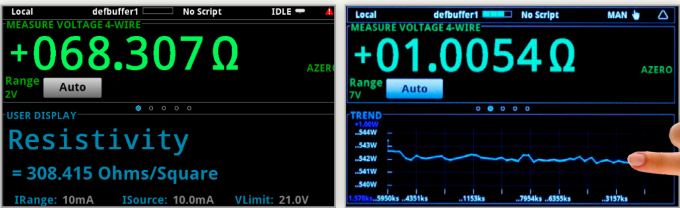
Modern instruments, such as Keithley's Model 2450 or 2460 Touchscreen SourceMeter® SMU Instruments, can display resistivity on the user interface.
