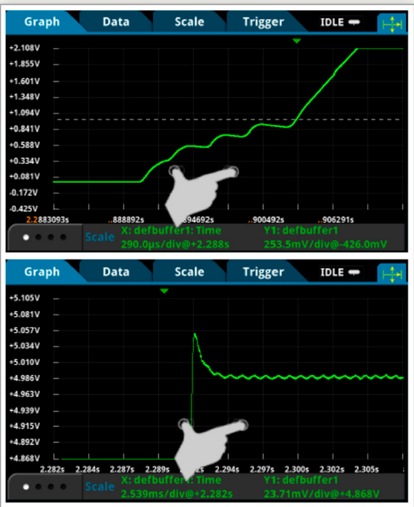
Panning and zooming into the soft-start behavior (top) and output voltage overshoot before reaching steady state (bottom.)
