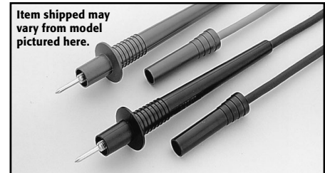
Model 1751 Safety Test Leads: 91.4cm (36 in) test lead set supplied with each Model 175A and 197A. Finger guards and shrouded banana plugs help minimize the chance of making contact with live circuitry.
